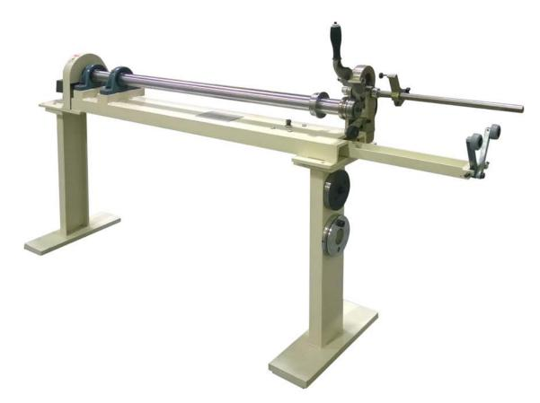
The Dusenbery<sup>®</sup> Model 765 AB Core Cutter provides an efficient method for precision cutting of cores with 3" to 6" ID and up to 90" long. Ruggedly built for low maintenance with a long lasting steel cutting platen. The platen may be easily shifted to different cutting positions to present a fresh cutting edge. Adapter ring assemblies, designed to accommodate a wide range of core sizes, are also quickly changed by removing a single socket head screw.
