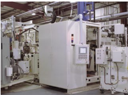
MDO Shown here between the casting machine and intermediate winder. The machine direction orienter was designed with an emphasis on process flexibility and features the patented CRD technology.
